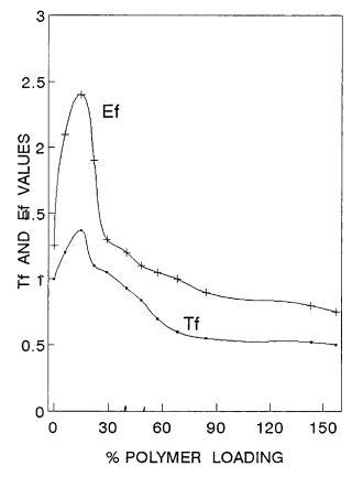
**Figure 4** Tensile strength of gamma-treated jute yarns against polymer loading with MMA.
