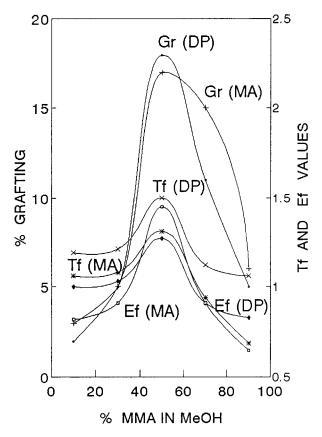
**Figure 7** Grafting and tensile properties of jute yarns treated under UV radiation at different MMA concentrations in the presence of MA and DP additives only.
