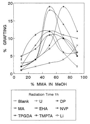
**Figure 6** Grafting of jute yarns with MMA in the presence of different additives.
