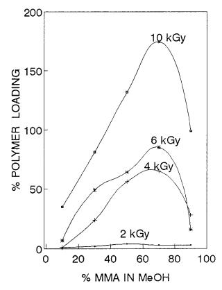
**Figure 2** Polymer loading versus MMA concentration as a function of total dose.
