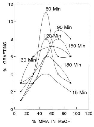
**Figure 5** Grafting of jute yarns with MMA under UV radiation at different irradiation periods as a function of MMA concentration.
