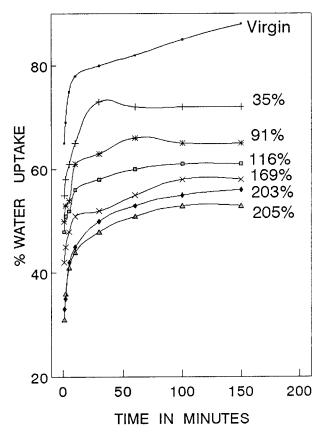
**Figure 8** Water uptake by treated and untreated jute yarns against soaking time.
