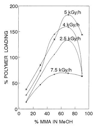
Figure 1 Polymer loading versus MMA concentration as a function of dose rate.
