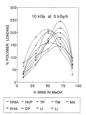
**Figure 3** Polymer loading with MMA in the presence of different additives.
